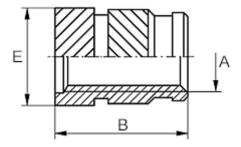
Female thread A = M10 Length B = 9.5 Min distance to edge = 4.0 Outer diameter E = 12.3 Recommended bore diameter W +0.1 = 11.7
